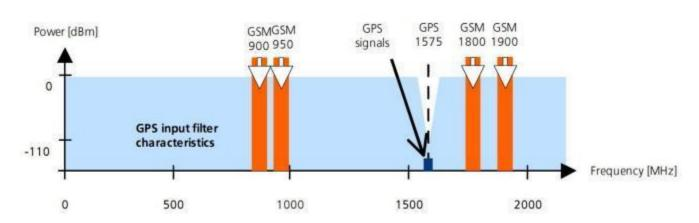
ST337G-18C43-DZ710 configured SAW to reduce the out-bandjamming by adding SAW filter.
